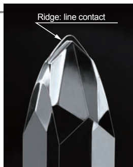
● Stylus model magnified 2000 times
